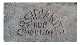
**Obsidianite** bricks got their name from Obsidian i.e. molten lava set solid from a volcano. These bricks were acid proof and would withstand exposure to all acids except fluorine. Ron recalls orders for obsidianite bricks by cement manufacturers to line the top of chimneys where acid formed and eroded traditional bricks.
